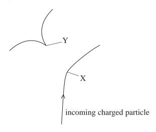
At X an incoming charged particle interacts with a stationary proton.
